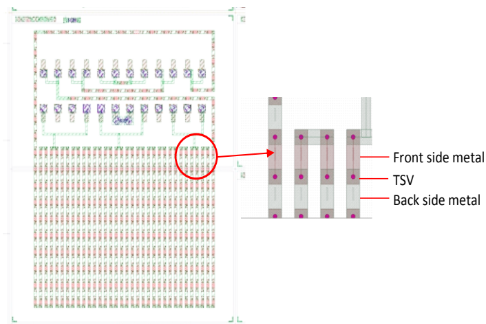
10x100 µm : 2 to 754 TSVs Daisy Chain
