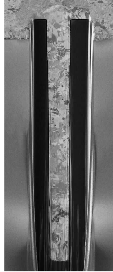
Option 2 MOCVD TiN – Flash Cu PVD 200 nm - 200 nm eG 3D seed
