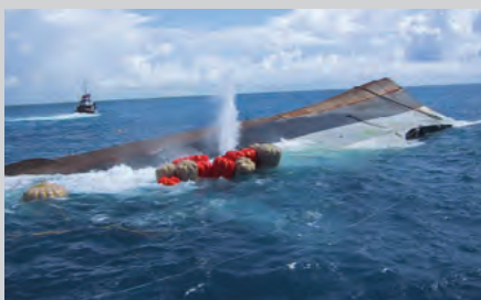
Raising the Spiegel Grove, a 510 ft U.S. Navy troop transport ship.
