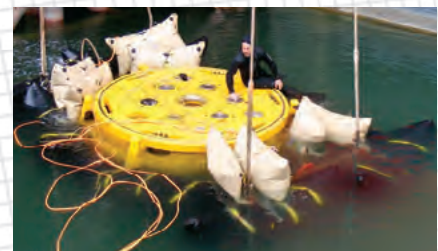
Lowering instrumentation using Enclosed Flotation Bags 500 lbs. and Enclosed Flotation Bags 6,000 lbs.
