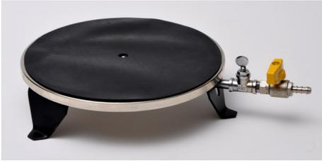
High Vacuum pump plate, Cast Iron, with Rubber Gasket, accommodates Bell Jars up to 8 1/2" DIA. equipped with shut off valve and bleeder valve
