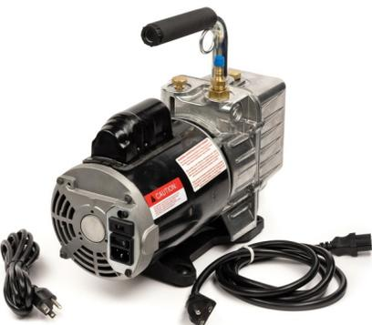
Rotary Vane High Vacuum Pump: 5cfm, 110V/220V, 60Hz/50Hz, with 0-30" Bourdon Tube Type Gauge, 1/2HP Comes equipped with both US110V and US220V cords and plug into the back of the motor. There is also a switch on the motor to easily switch between voltages.
