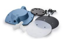
PILOT Service Kit - Major Rebuild Parts TLD5000 - Includes Diaphragm Buna N, Diaphragm Liner PTFE, Diaphragm Hold Down Plate, Valve Plate Assembly, O-Ring Gasket Head, Pump Head Assembly, Head Screws, Handle Screws, Diaphragm Hold Down Screws & Hose Barb PVDF 1/8" x 1/4" ID Hose.
