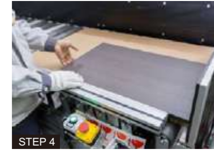
STEP 4 Put the panel in the middle
