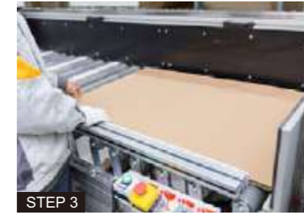
STEP 3 Place honeycomb-paper cardboard at the bottom
