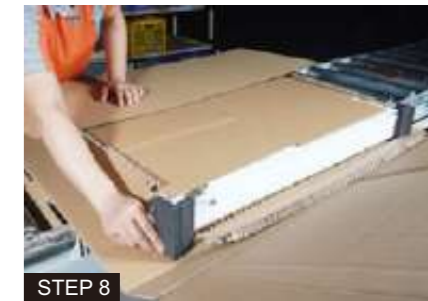
STEP 8 Fill with honeycomb-paper cardboards, protect the four corners with EVA foam
