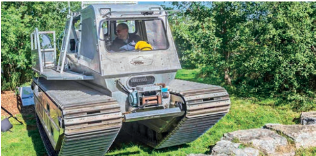
A Marsh Master can be used to shred phragmites.
