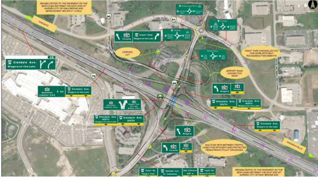
A visual of the diverging diamond interchange. SUPPLIED
