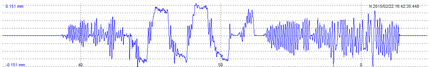
oscillogram in absolute displacement of the vibrating table
