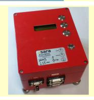
The AceBox is an high performance accelerograph. Based on the powerful SL06 recorder it embeds three force balance accelerometers capable to record the seismic signal at high resolution in standard USB flash pen drives.
