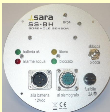
Picture of the control panel with LEDs for battery check, lock-unlock switch and status, wet alarm, battery connector, sensor connector and fuse.
