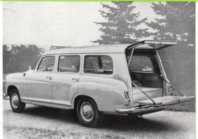
Station car with rear flap door
