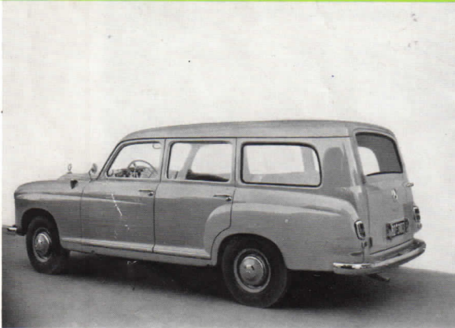
Station car with rear wing door
