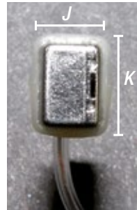
Symbolic image 17 High Power receiver I = 10 \text{ mm} , J = 4.5 \text{ mm} , K = 5.5 \text{ mm}
