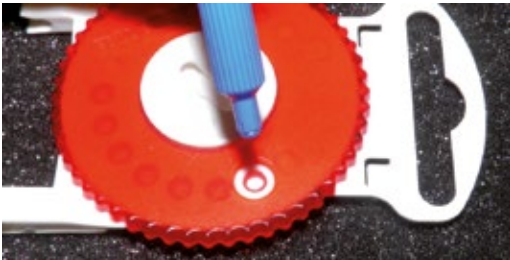
Removing the HF3 filter
