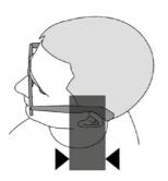
Also ensure that the device's temple does not come into contact with the skull (Fig. 4.3.4), as this may impair both the sound quality and speech intelligibility, and mechanical feedback may occur. This can be avoided by further bending the spectacles.
