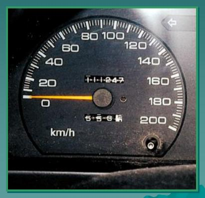
speedometer measures the instantaneous speed of the car
