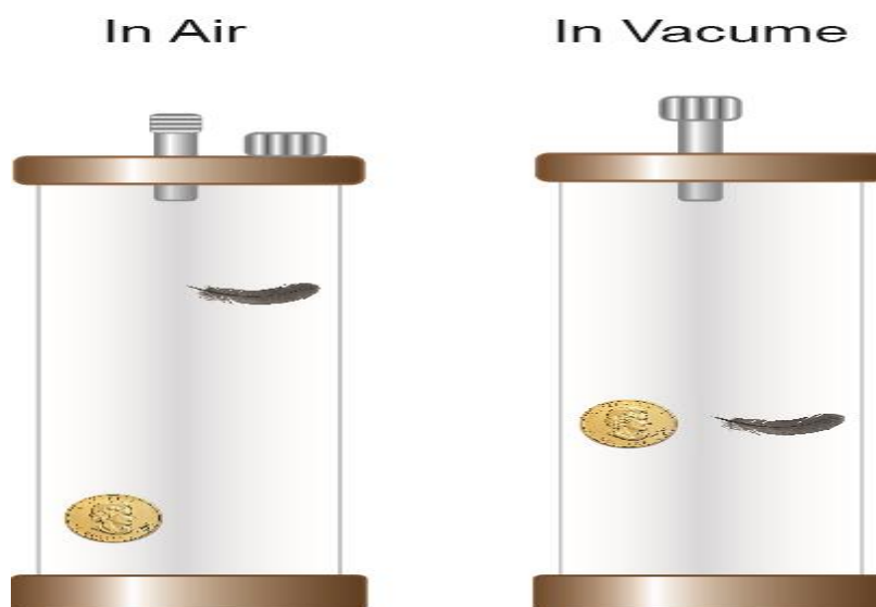
Figure-4. Comparison of free fall of a feather and a coin demonstrated by a physical setup
