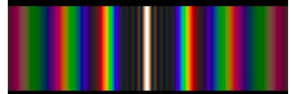
Interference pattern of white light through a grating
