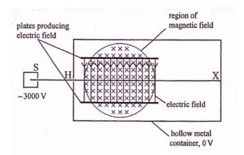
Upon entering the casing, the negative ions enter a region in which a magnetic field of flux density 0.83 T and an electric field of field strength *E* are applied at right angles to each other. The negative ions continue moving with constant velocity in a straight line through the fields.
