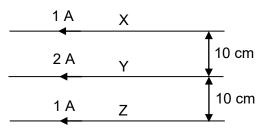
[Magnetic flux density due to long straight current-carrying conductor is  $B = \frac{\mu_0 I}{2\pi r}$ ]
