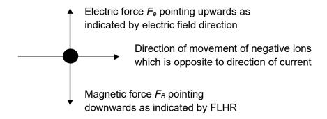
Hence, when the two forces are equal in magnitude, and the vertical resultant force is zero, the ions will move through without deflection.
