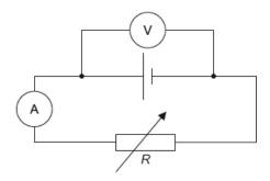
The variable resistor is adjusted and a series of current and voltage readings are taken. The graph shows the variation with  ${\cal R}$  of the power dissipated in the cell and the power dissipated in the variable resistor.
