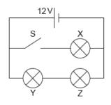
2a. The switch S is initially open. Calculate the total power dissipated in the [2 marks] circuit.
