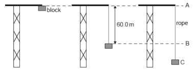
The unextended length of the rope is 60.0 m. From position A to position B, the block falls freely.
