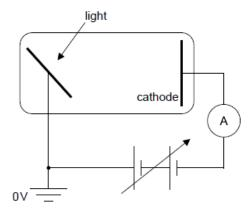
The graph shows the variation of the current  ${\cal I}$  in the ammeter with the potential  ${\cal V}$  of the cathode.
