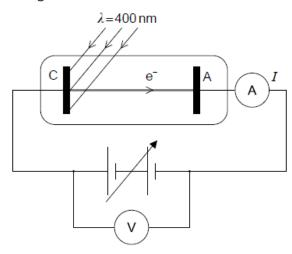
12a. A current is observed on the ammeter when violet light illuminates C. [3 marks] With V held constant the current becomes zero when the violet light is replaced by red light of the same intensity. Explain this observation.
