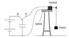
When the switch is connected to X, the capacitor is charged using the battery. When the switch is connected to Y, the capacitor fully discharges through the electric motor that raises a small mass.
