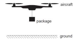
The air is propelled vertically downwards with speed v. The aircraft hovers motionless above the ground. A package is suspended from the aircraft on a string. The mass of the aircraft is  $0.95\,\mathrm{kg}$  and the combined mass of the package and string is  $0.45\,\mathrm{kg}$ . The mass of air pushed downwards by the blades in one second is  $1.7\,\mathrm{kg}$ .
