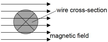
The wire which carries a current of 3.5A into the page, is placed in a region of uniform magnetic field of flux density 0.25T. The field is directed at right angles to the wire.
