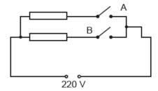
The circuit transfers 1.6 kW when switch A only is closed. The external voltage is 220 V.
