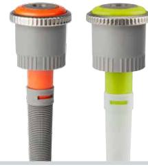
**Bold** = Optimal pressure for the MP Rotator is 40 PSI. To achieve the lowest radius setting of 6', it will be necessary to regulate the inlet pressure to 30 PSI. Pair with Pro-Spray® PRS30.
