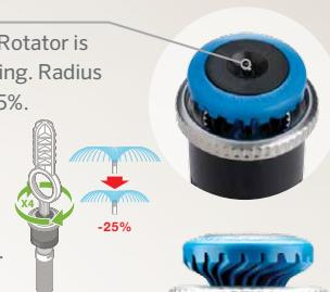
**Arc Adjustment Ring** Install the MP Rotator with the Left Edge Indicator aligned with the left edge of the landscape. The MP Rotator not only features a fully adjustable arc, but as the arc is changed, the flow adjusts proportionally to maintain matched precipitation.
