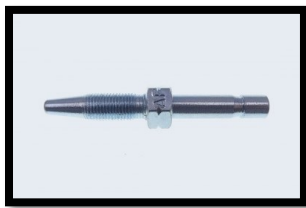
100-054-NUT-SW | SE&T | HOSE STUD STRAIGHT GROOVED, BLACK | D 6 | L 52,5 | L1 21,5 | HOSE Ø 4
