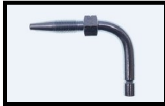
3511-116 | SE&T | HOSE STUD 90° GROOVED, BLACK | D 6 | H 17 | L 28 | HOSE Ø 4
