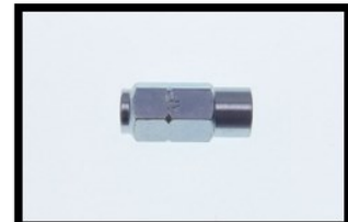
100-050 | SE&T | SCREW SLEEVE | L 28 | SW 12 | HOSE Ø 4
