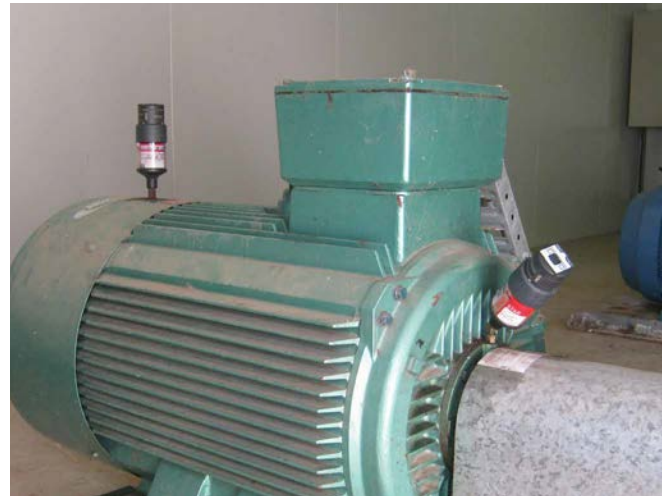
Application Electric motor Lubricator perma STAR VARIO 120cm 3 Installation kit Direct mount
