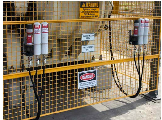
Application Conveyor pulley bearings and seals Lubricator perma STAR VARIO 500cm 3 Installation kit K265CX
