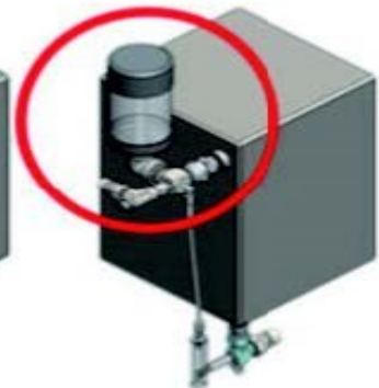
Side mounted breather connects vent line to bottom mounted drain mount Use "B"
