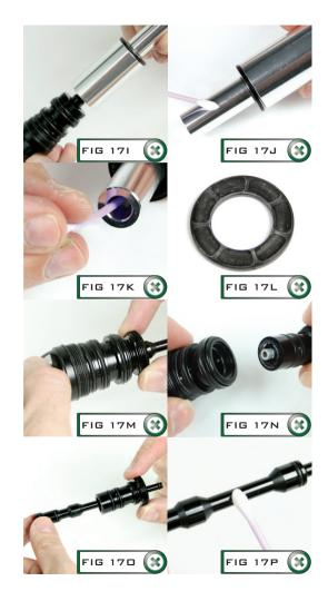
Moving onto the valve body: clean the three o-rings and the valve body itself (SEE FIGURE 170). Inspect the o-rings and internal bore of the valve body for damage and wear. Replace the o-rings as necessary. Inspect the two sets of air ports labelled A in FIGURE 170, making sure all the ports are free of any debris.
