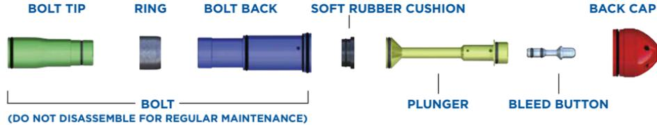
The SLG™ BOLT is the main component of the SLG™ marker. In order to achieve the best possible performance, it is essential that the SLG™ BOLT is kept clean, well lubed and in good working order.
