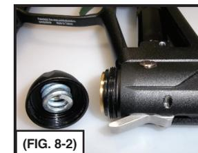
2. Flip the On/Off Lever forward to Off position. Insert the 1/2in. hex socket into open side of Regulator and unscrew the brass nut from the Regulator in the counter-clockwise direction (Fig 8-3).
