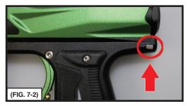
While holding the button, grip and pull the Bolt Guide free of the Body removing the bolt system (Fig 7-3)
