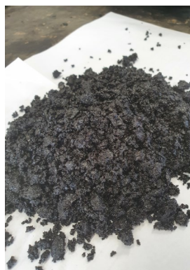
approx. 113 Tonnes of Recycled Asphalt Pavement (RAP)
