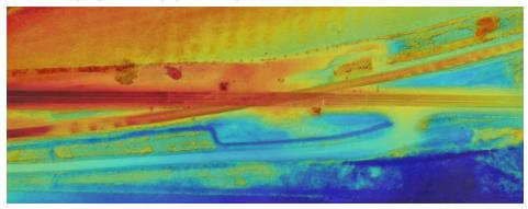
**Conclusion :** Drones mapping of rail corridors has emerged as a reliable and faster alternative to ground based surveying and mapping which can be expensive and time consuming. Orthorectified images are geometrically corrected so the scale is uniform throughout the digital image hence allows linear and volumetric measurement on computer screens without site visits.
