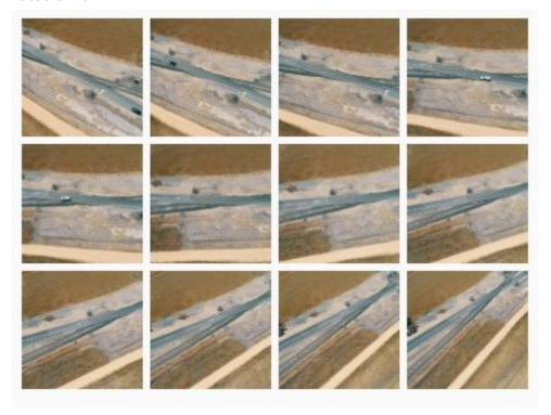
3. Orthorectified map - All images are stitched and orthorectified using dronedeploy and Pix4D platforms.
