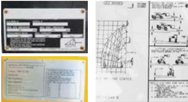
Examples of compliance plates and load charts for telehandlers.
