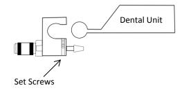
Tighten set screws of hanger mount onto dental unit ½" bar.
