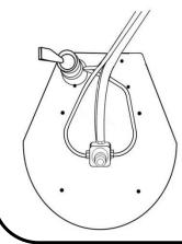
If the existing foot pedal does not have a toggle switch, install a toggle switch as shown. Utilize constant air flow from the foot pedal manifold to supply the toggle switch. If the foot pedal already has a toggle switch, skip this step.
