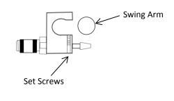
Tighten set screws of hanger mount onto swing arm ½" bar with allen wrench.
