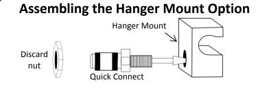
Remove the nut from the quick connect and discard. Thread quick connect into the hanger mount with 12 mm wrench.
