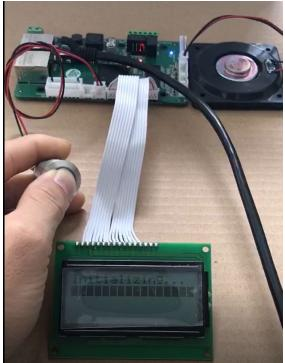
IMAGE: Two Pin Short using a push button as an example
