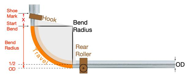
X = Distance between Shoe Mark and Start Bend Start Bend = Bend Radius + 1/2 OD
