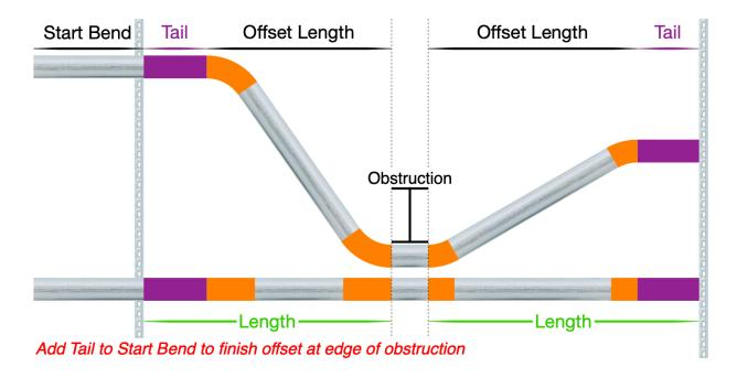
Bend Aid does not solve saddles directly, use the other solutions and layout two offsets on one section of conduit.
