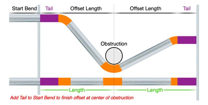
Bend Aid does not solve saddles directly, use the other solutions and lay out two offsets on one section of conduit.
