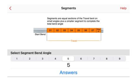
Segments are equal sections of the Travel bent on small angles plus a smaller segment to complete the total bend angle
