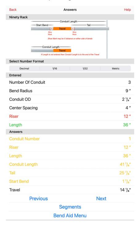
The center to center spacing must be greater than the Conduit OD.
