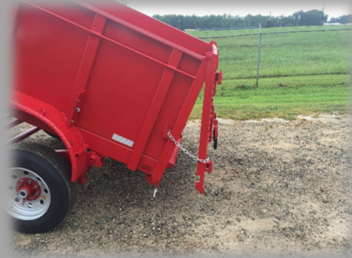
REAR BARN DOOR & SPREADER COMBO GATE
