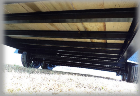
3" CHANNEL CROSSMEMBERS 16" OC 7" CHANNEL MAIN FRAME
