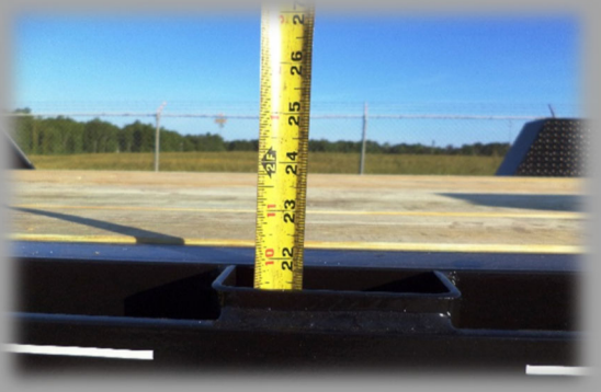
22" DECK HEIGHT – 4" DROP AXLES
