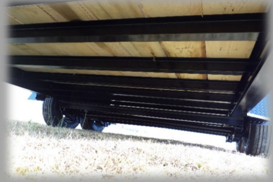
3" CHANNEL CROSSMEMBERS 16" OC I-BEAM MAIN FRAME
