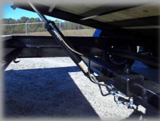
HYDRAULIC GRAVITY FEED CUSHION CYLINDER W/ CONTROL SPEED
