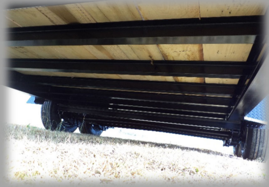
3" CHANNEL CROSSMEMBERS 16" OC 8" CHANNEL MAIN FRAME
