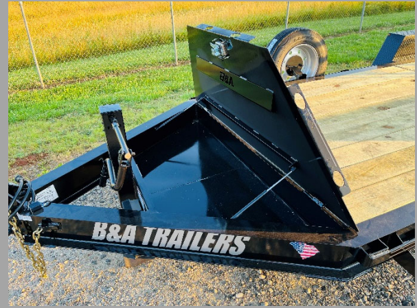
HD CHECKER-PLATE TONGUE LID ALLOWS EXTRA DECK SPACE & AMPLE STORAGE
