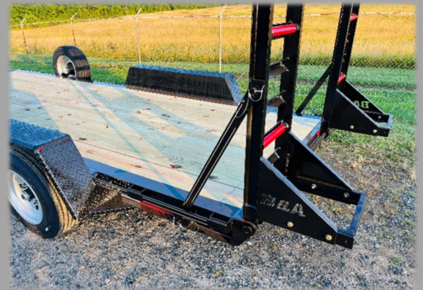
I-BEAM FRAME, HD CHECKERPLATE FENDERS, SPRING ASSIST RAMPS
