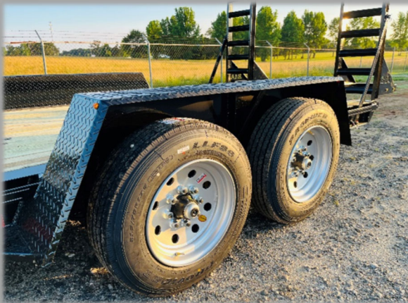
I-BEAM FRAME, HD CHECKERPLATE FENDERS, SPRING ASSIST RAMPS
