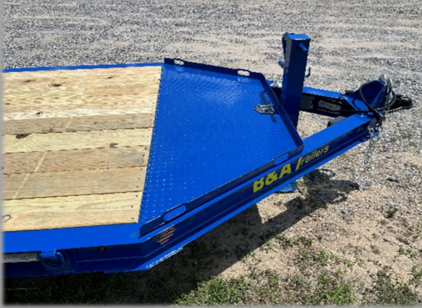
HD CHECKER-PLATE TONGUE LID ALLOWS EXTRA DECK SPACE & AMPLE STORAGE
