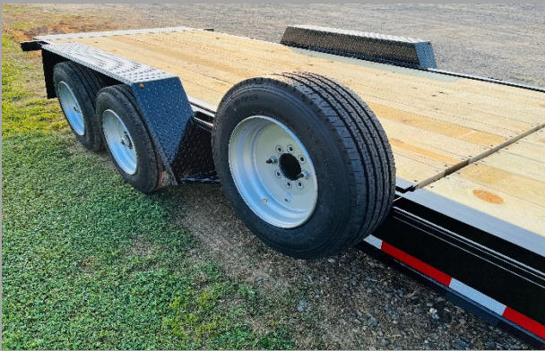
EASY LOAD ANGLE, 8K AXLES W/ 12 1/4" X 3 3/8" ELECTRIC BRAKE, 215 75 R 17.5 (16 PLY) RADIAL TIRES
