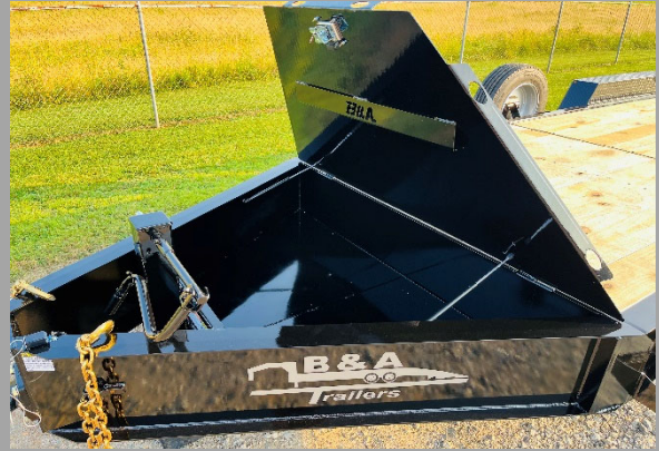
HD LOCKING TONGUE LID W/ GAS STRUT SHOCKS & DEEP WELL BOX PROVIDES AMPLE STORAGE & VALUABLE EXTRA DECK SPACE
