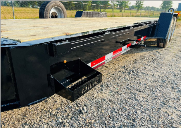
HD ONE PIECE 12" BEAM FRAME DESIGN W/ BOARDING STEP AND HD CHECKERPLATE FENDERS
