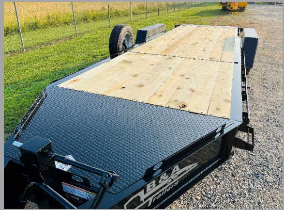
HD ONE PIECE 12" BEAM FRAME DESIGN W/ BOARDING STEP AND HD CHECKERPLATE FENDERS
