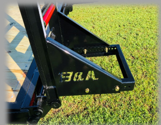
SPRING-ASSIST RAMPS ADJUSTABLE GROUND SUPPORTS
