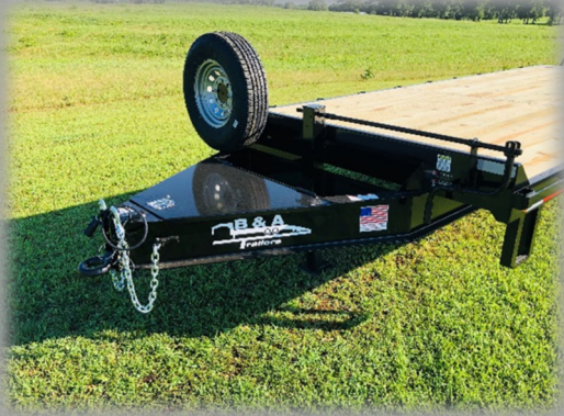
TOOL TRAY W/ LOCKING LID, SPARE TIRE 12K JACK, BOARDING STEP
