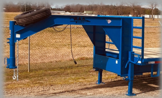
GOOSENECK PACKAGE AVAILABLE CROSSMEMBERS 16" ON CENTER
