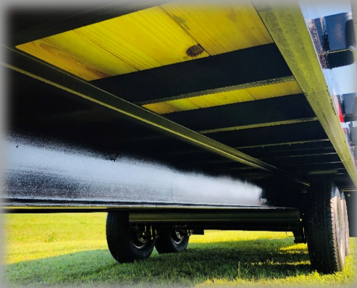
10" I-BEAM W/ 16" CENTER CROSS-MEMBER FULL-LENGTH RUB RAIL & STAKE POCKETS
