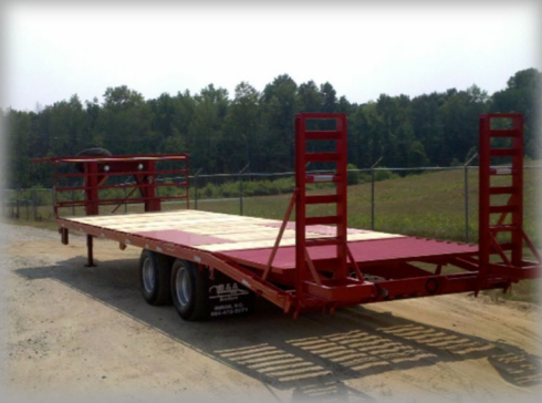
12" I-BEAM FRAME – 102" WIDE – 34" DECK HEIGHT
