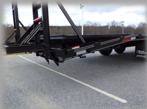
FLIP-UP BEAVERTAIL (OPTION) FULL-LENGTH RUB RAIL & STAKE POCKETS
