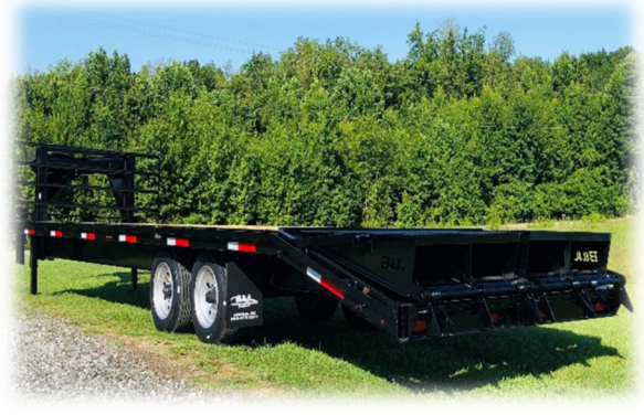
FULL-WIDTH "B&A JUMBO RAMPS™" OPTION SPRING ASSIST
