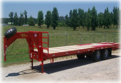
12" I-BEAM FRAME – 102" WIDE 34" DECK HEIGHT
