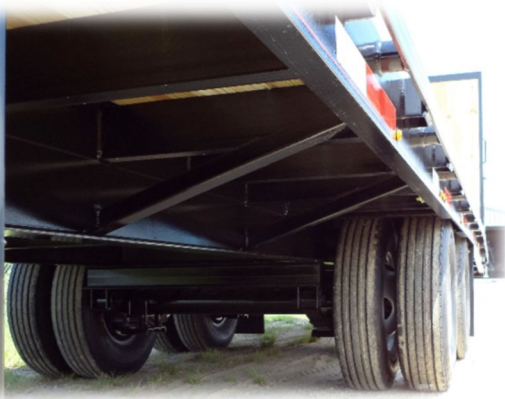
LOW-PRO PIERCED FRAME DESIGN FULL-LENGTH RUB RAIL & STAKE POCKETS
