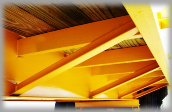
12" PIERCED FRAME, 3" CHANNEL CROSSMEMBERS 16" ON CENTER
