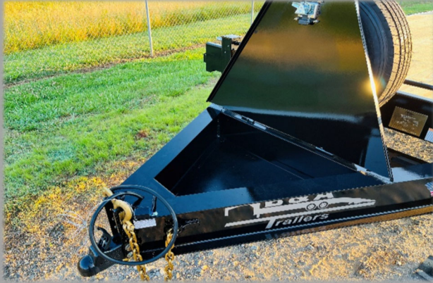
Locking tongue box w/ solid floor, Dual jacks, Adjustable 21K Demco Coupler
