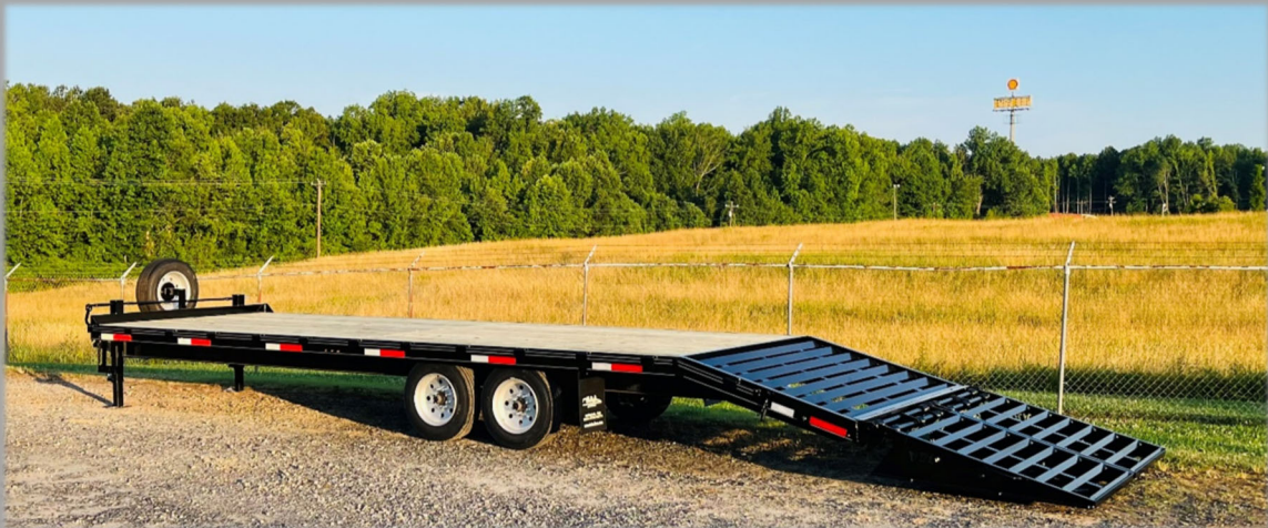
Easy full-width load angle, I-Beam Frame, 102" width, 8K axles, 16 ply tires
