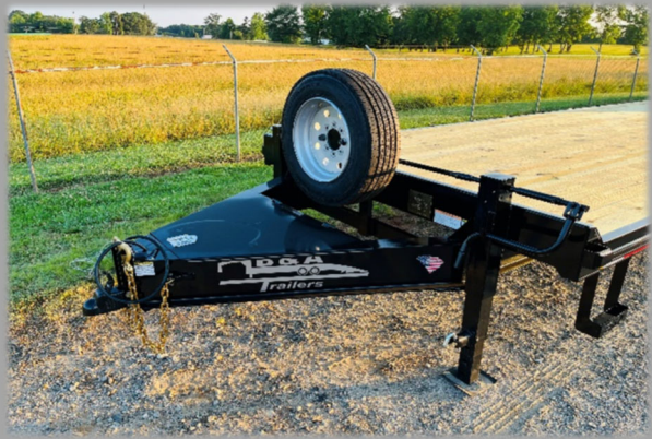
Locking tongue box w/ solid floor, Dual jacks, Adjustable 21K Demco Coupler
